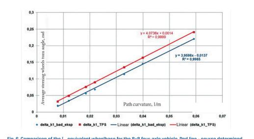
Fig. 6. Comparison of the  $\rm L_e$  equivalent wheelbase for the 8×8 four-axle vehicle. Red line - course determined with the use of formula (7). Navy blue line - course determined on the basis of the experimental tests data
